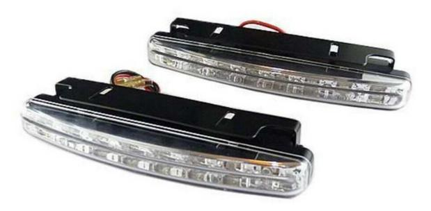
The mounting plate sits on top of the light in the illustration but can be rotated. I twisted it ninety degrees and turned the light over so the plate protrudes below the light. I made up an inverted "J" or hook shaped bracket. Drilled a hole in the short leg for the outer bolt on the bumper bar mounting bracket. I used some scrap aluminum strip 50mm x 3m I had bought at Bunnings for reasons I have long forgotten.
